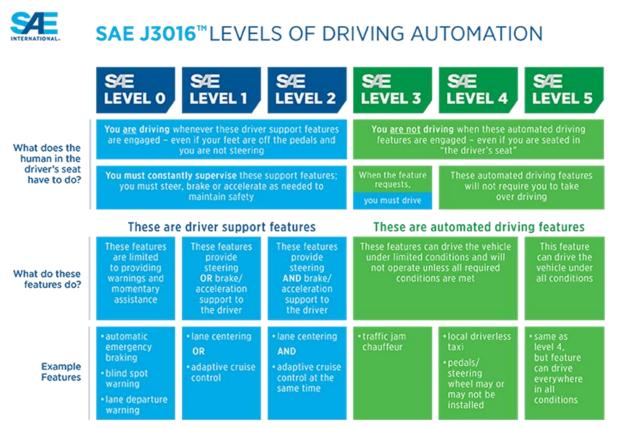
Figure 1. Levels of driving automation [1]
